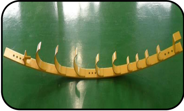
➤ Pipe Supports/ Hangers
